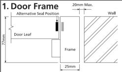
The frame to wall gap must be filled with stone wool or sealed with intumescent mastic if less than 6mm wide.
